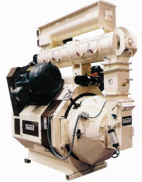
**Figure 5.** A compression pelleting machine
