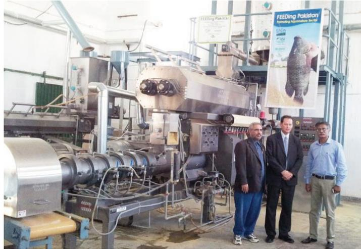
**Figure 6.** E-750 extruder machine with accessories.
