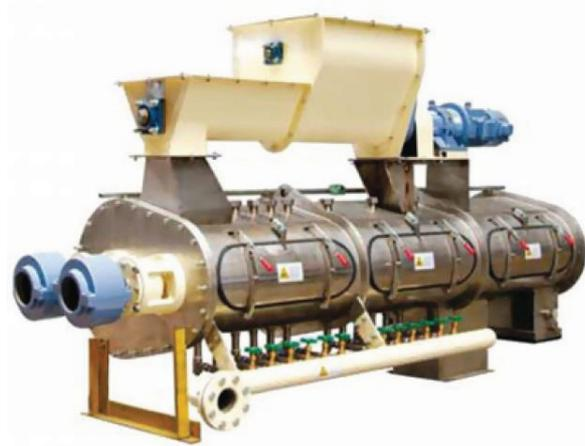
Figure 9. A pre-conditioner with feed hopper
