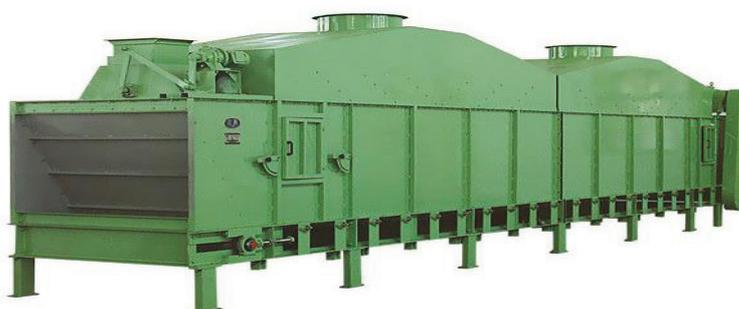
Figure 11. A horizontal belt cooler
