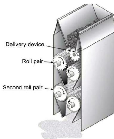
**Figure 3.** Grinding process is a roller mill
