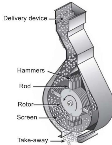
**Figure 2.** Internal view of a hammer mill
