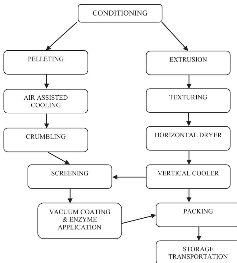
**Figure 1.** Flow Diagram of Aqua Feeds Manufacturing Processes.
