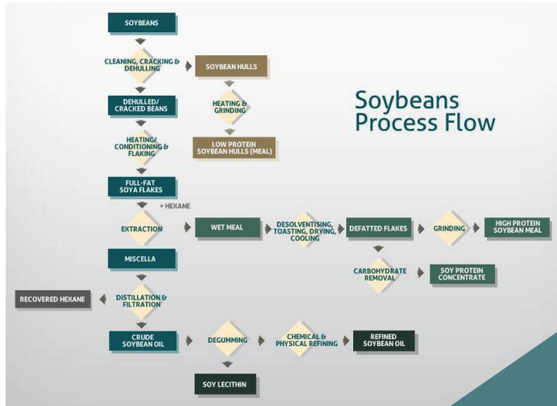
Figure 6. A schematic of the steps in soybean processing
