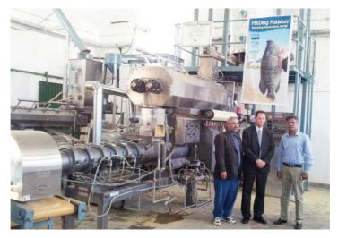
Figure 6. E-750 extruder machine with accessories.
