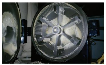
Figure 4. A typical Pulverizer for fish feed production
