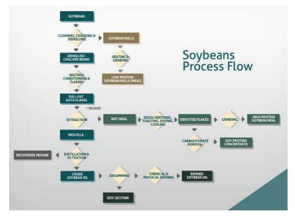
Figure 6. A schematic of the steps in soybean processing *Source:* Wilmar International, Singapore
