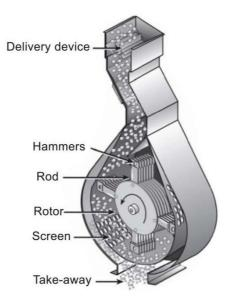
Figure 2. Internal view of a hammer mill
