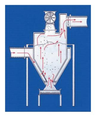
Figure 10. Air flow in a vertical cooler
