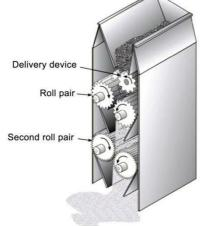
Figure 3. Grinding process is a roller mill
