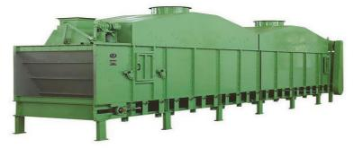
Figure 11. A horizontal belt cooler
